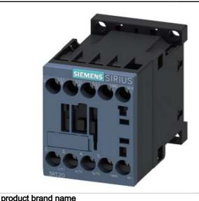
CONTACTOR, AC-3, 7.5KW/400V, 1NO, DC 24V, 3-POLE, SZ S00 SCREW TERMINAL .
